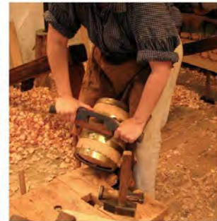
Buzz—cleans up the outside surfaces.
