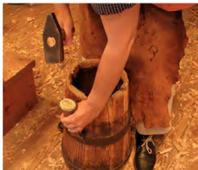
Hammer and Hoop Driver—tap the hoops into place.
