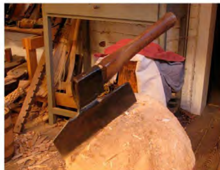
Broad Axe—rough-shapes the bevels on the staves.
