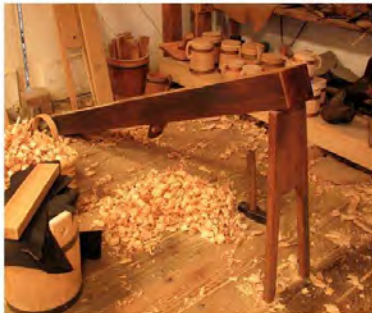
Jointer Plane—shaves the bevels and creates the tapers on the staves.
